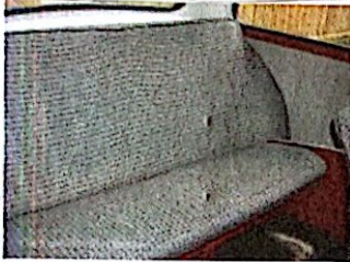
The rear seat is also plain and little more than a bag over the padding. The rear wheel arch is also covered.
