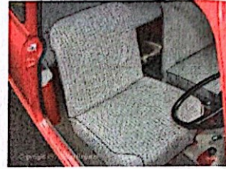
Basic seats were of cloth material. These are 59 style basic seats of the correct pattern. Black piping indicates a Morris.
